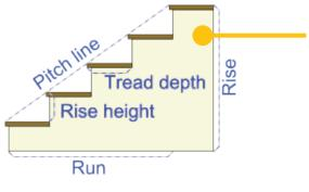
A typical staircase and terms used to describe the various sections.
